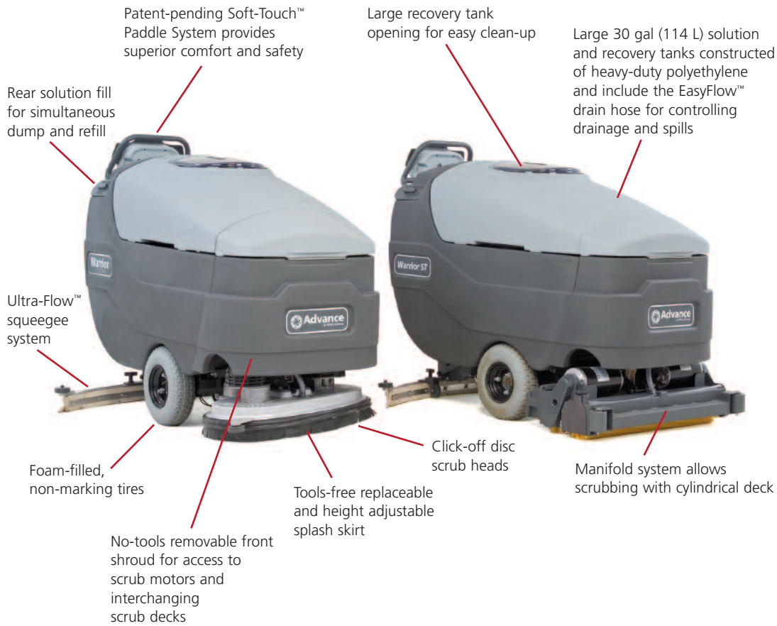
Warrior AXP scrubber includes a standard onboard battery charger for wet or gel battery packages.
